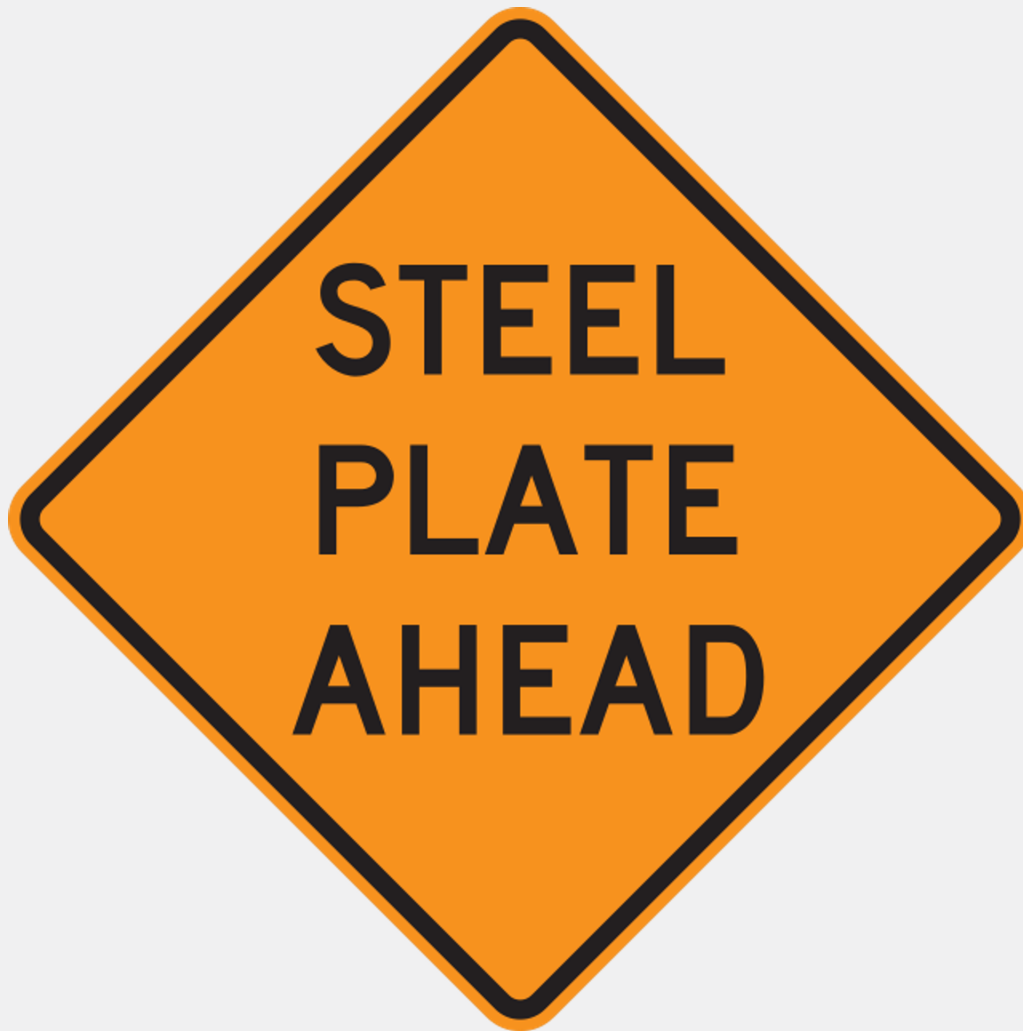
W8-24 Steel Plate Ahead
