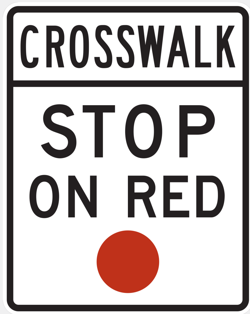
R10-23 Crosswalk — Stop on Red
