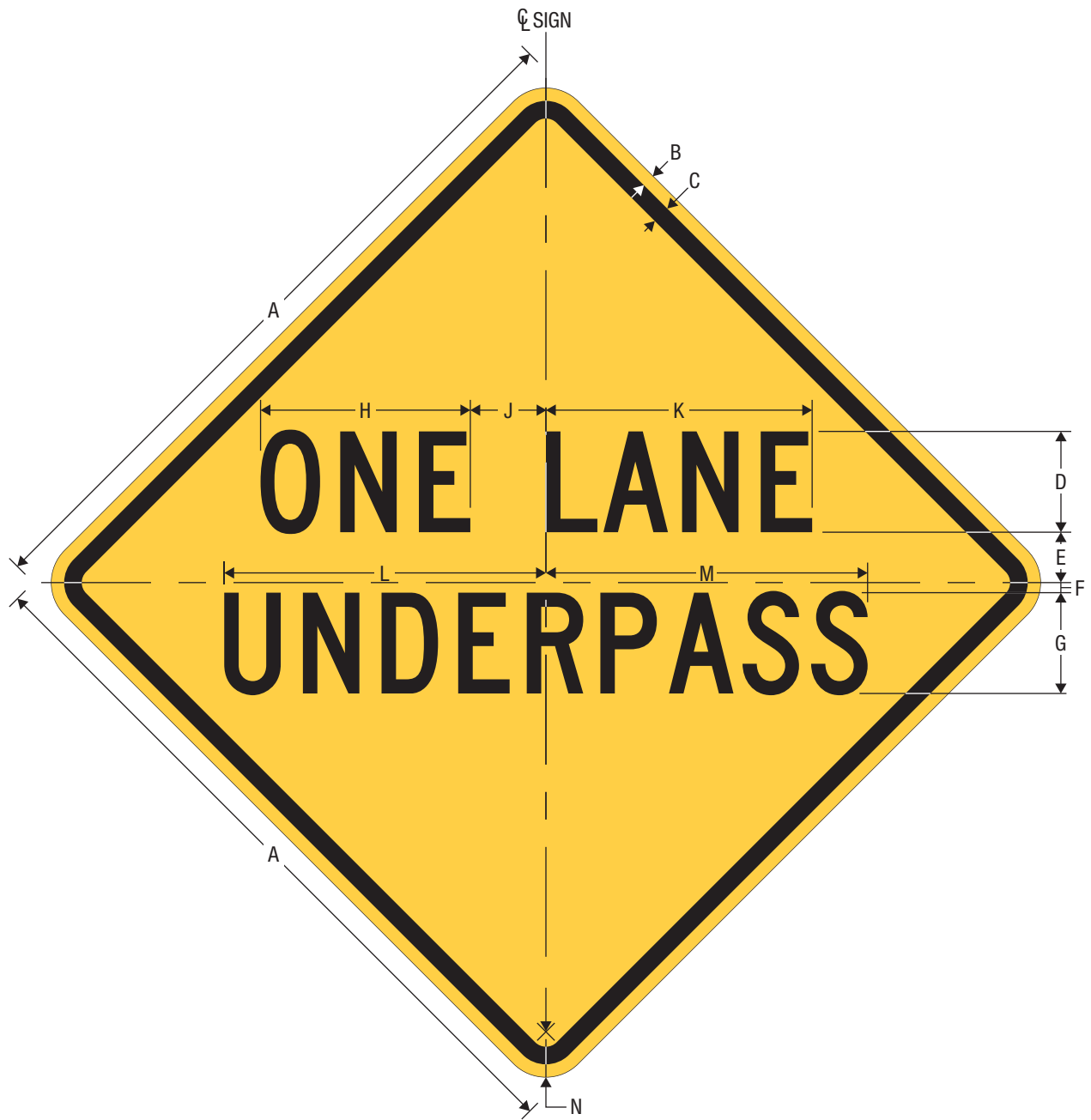
W5-3a ONE LANE UNDERPASS
