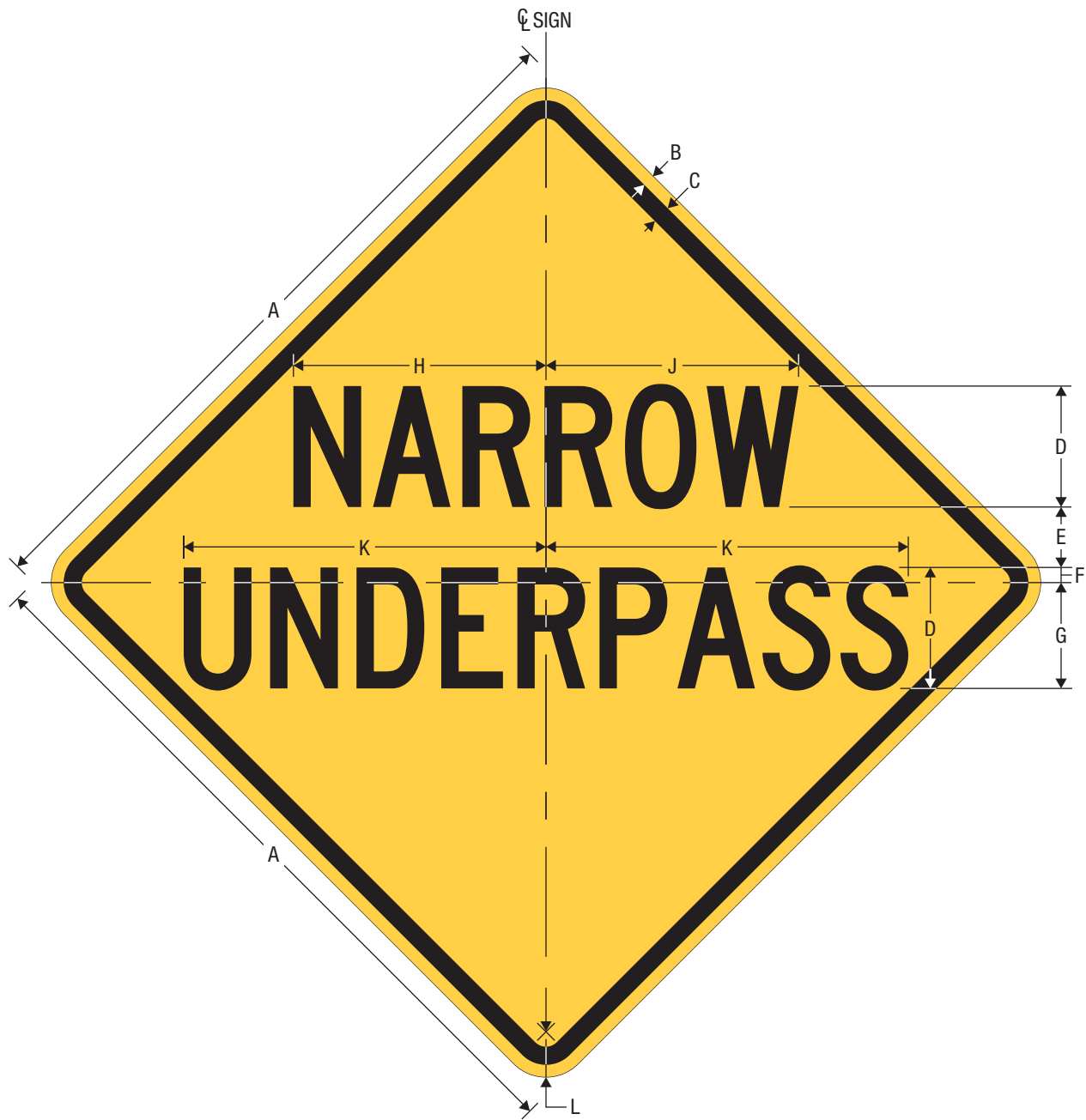
W5-2a NARROW UNDERPASS
